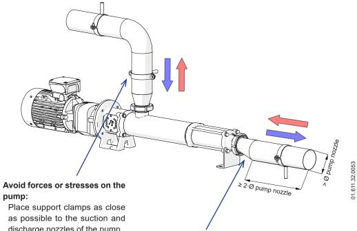
Place support clamps as close as possible to the suction and discharge nozzles of the pump. Expansion seals can be fitted between the pump and the suction/discharge pipes to absorb potential product volume changes, reduce mechanical stresses and reduce noise from vibrations.
