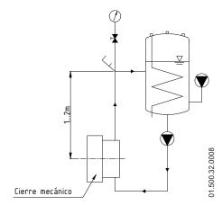
Auxiliary fluid pipes are recommended to be made of stainless steel and as short and straight as possible so that the auxiliary fluid can flow easily.
